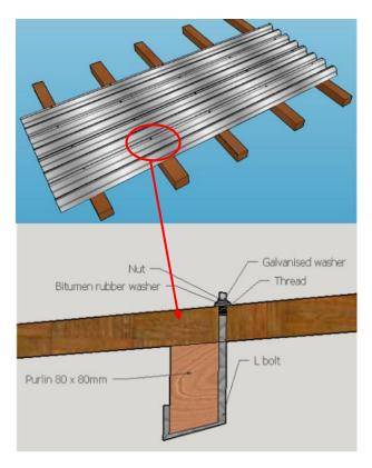
Fig.11 Sheeting to purlin connection detailings.
