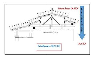
Fig. 7 Net force difference on a Drangim roof
