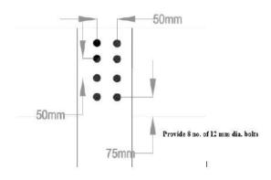
Fig.14 Lower strut to Dhingri connection detailings.
