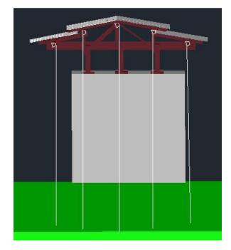
Fig.16 Tension Cable connection from the roof ridge
