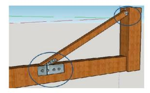
Fig.15 Inclined strut connection points
