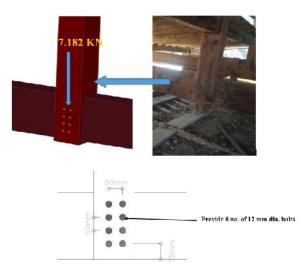
Fig.13Vertical struts to Dhingri connection detailings
